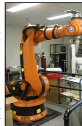
Robotic testing system to assess knee joint function at the MSRC led by Dr. Savio L-Y. Woo.
